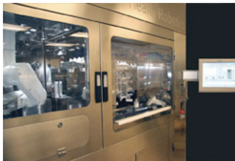
The robotic workbench is about 7-ft. wide, 6-ft. high, and 3-ft. deep. At left is the dose-preparation area with the robotic arm at rest. To the right is the loading chamber and the user's touchscreen. Photo courtesy of University of Colorado Hospital
