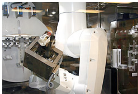
The robotic arm shows an ampicillin vial after reconstitution so that a pharmacy technician or pharmacist can visually
